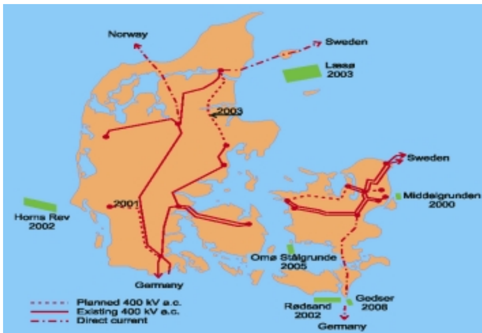
Fig. 3.11: High-voltage grid of Denmark [ www.Eltra.dk ].
